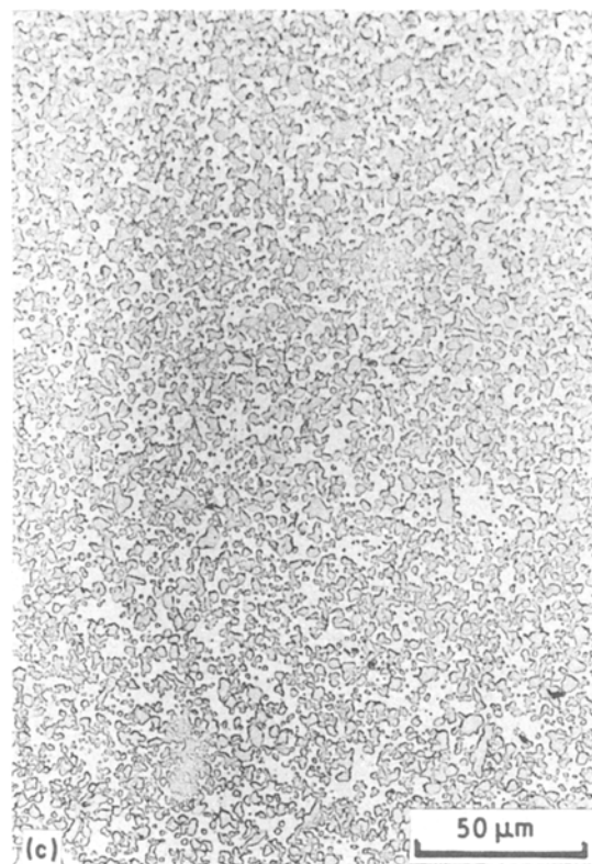
Figure 2 (a) Appearance of sample FM obtained through the rocket flight experiment, and the microstructures of samples (b) GM and (c) FM [1]. Sample GM was prepared on the ground.
